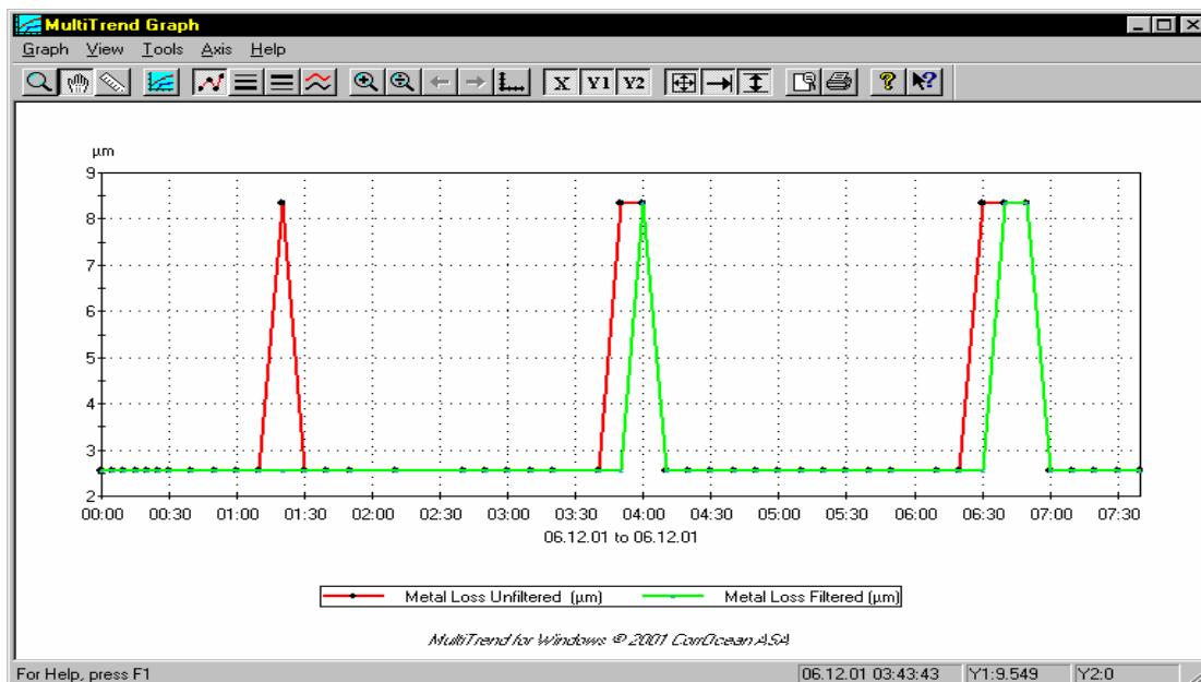
Figure 118118 Spike widths 2 Green signal is filtered
