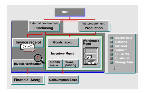
Material is procured from external or internal sources on the basis of the requirements determined by Material Requirements Planning. The delivery is entered in Inventory Management as a goods receipt. The material is stored (and managed under Inventory Management) until it is delivered to customers (Sales & Distribution), or is used for internal purposes (for example, for production).
